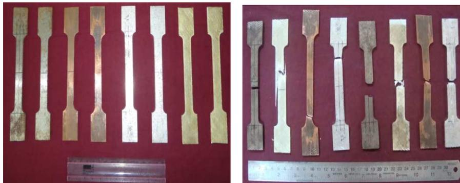
Figure 5: Un-Notched Tensile Specimens of GFRP, Al, Cu and HCS (Before and After Testing)
