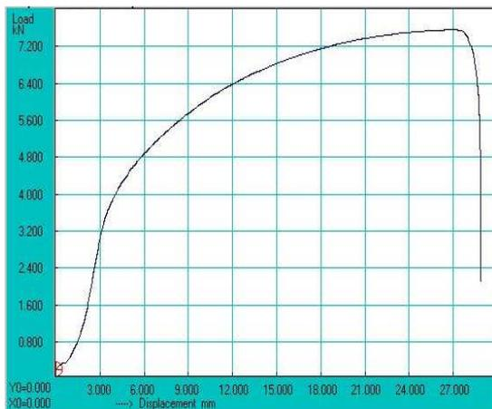
**Figure 6 (c): Cu Specimen**
