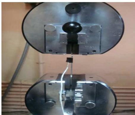
Figure 3: Details of AE Sensor Mounting
