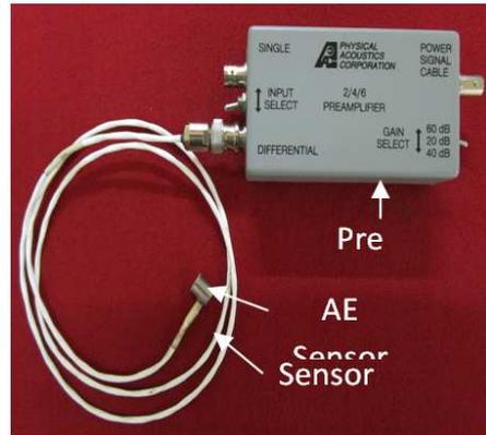
Figure 2: PAC AE Sensor with Pre-amplifier
