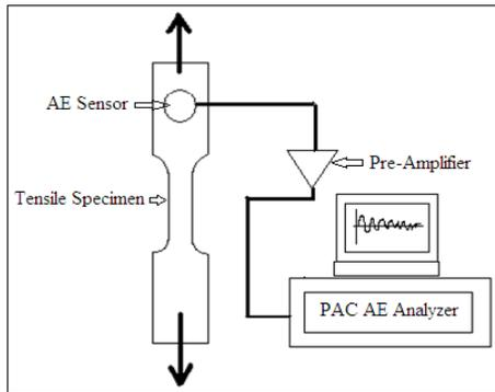
Figure 1 AE Data Acquisition Setup
